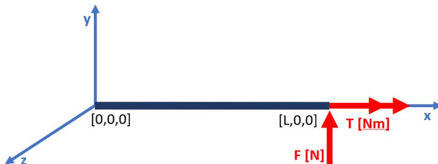
Fig. 1. Cantilever beam loaded with bending (bending force F) and torsion (torque moment T)
