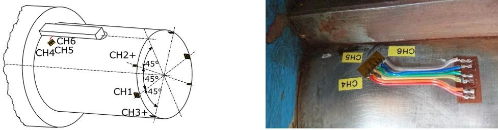
Fig. 2. The scheme of the location of the installed strain gauges (left) and detail of the strain gauge rose at the crack tip (right)
