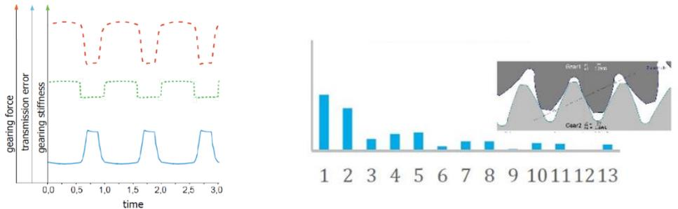
Fig. 4. (a) Example of periodic gear mesh excitation (b) Fourier coefficients
