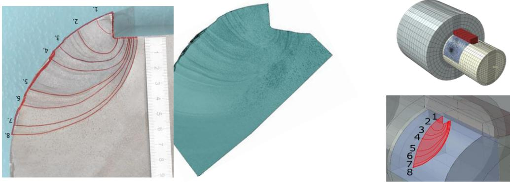
Fig. 4. The fractographic reconstruction of the crack front in different damage time and FEM model geometry for selected crack lines for calculation of the SIF and geometric correction functions [2]
