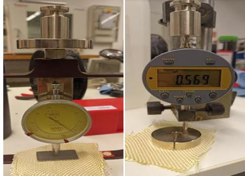
Fig. 1. Fabric thickness measurement setup (a) analogue, (b) digital
