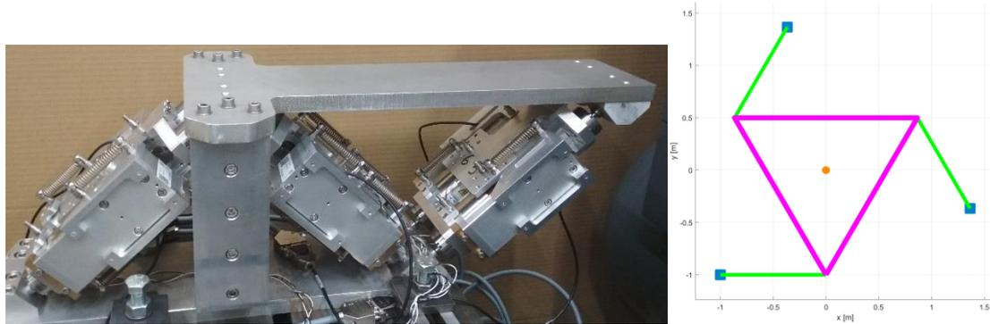
a) Perpendicular design of 3-DoF absorber      b) Symmetrical design of 3-DoF absorber
