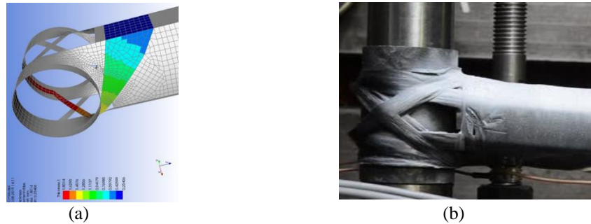
Fig. 2. Finite-element model (a); real part of the integrated composite joint at the end of a carbon fibre composite rod (b)
