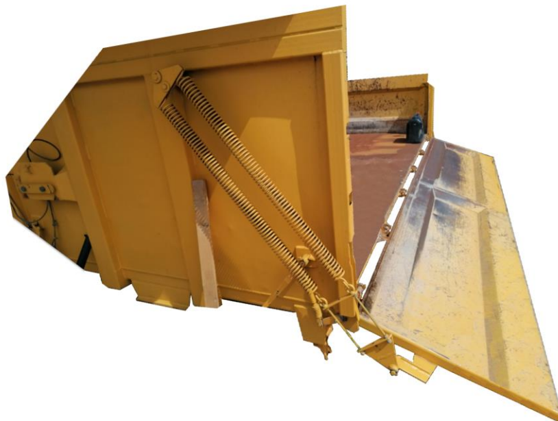
Fig. 1. Tipper body with spring mechanism, opened sidewall
