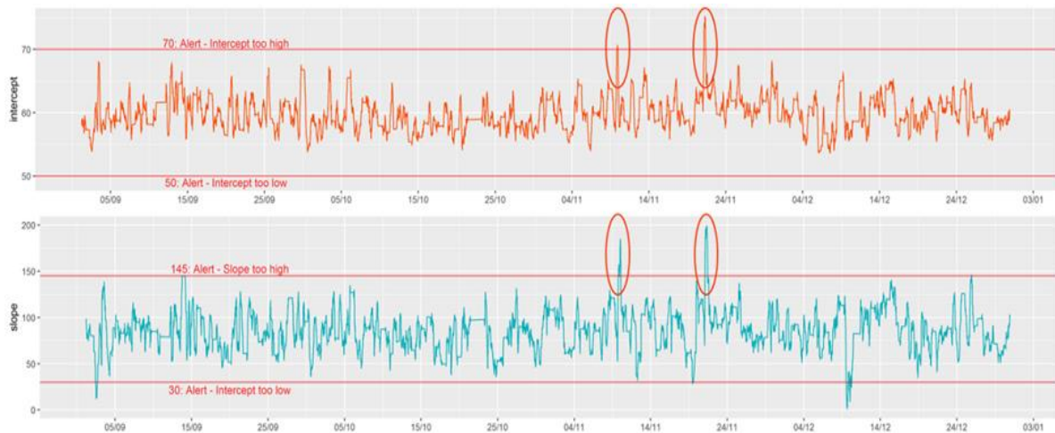
Fig. 3. Intercept and slope in a robust linear model estimated within a four-hour sliding window
