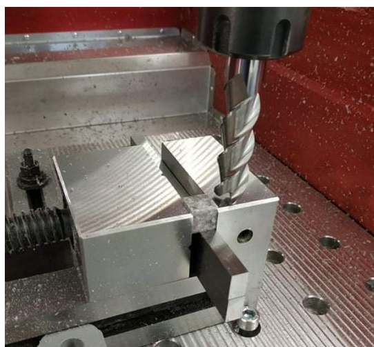
Fig. 1. Machining a foam specimen
