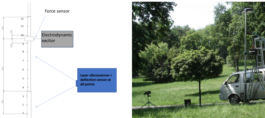
Fig. 2. Measurement setup for experimental modal analysis of lighting poles
