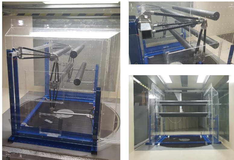
Fig. 2. Experimental set-up with mounted cylinders represented a real configuration of hangers
