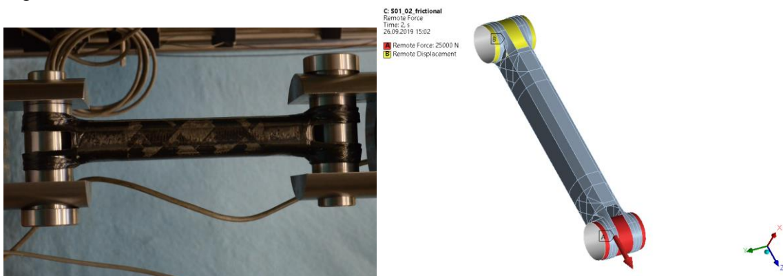
Fig. 1. Composite coupon with integrated loops and its model
