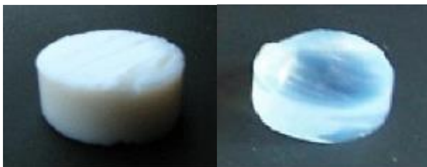
Fig. 2. Swollen macroporous gels – macroscopic appearance of tested sample
