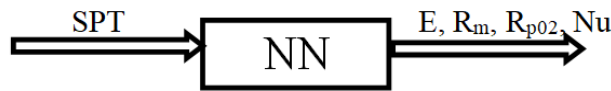
Fig. 1. Diagram of the program, where E = Young's modulus of elasticity, R_{p02} = yield strength, R_m = strength limit and Nu = Poisson number
