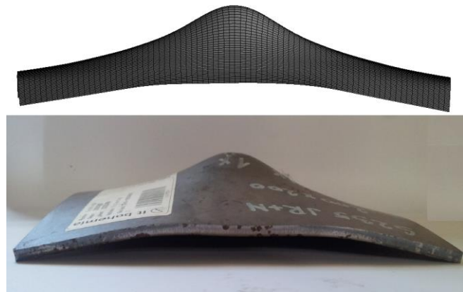
Fig. 2. The comparison of simulation and experiment with flat 200x200 mm 200g of TNT
