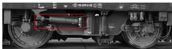
Fig. 1. Yaw damper on locomotive
