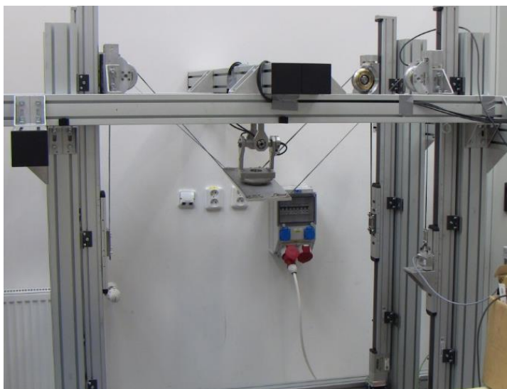
Fig. 1. The QuadroSphere tilting mechanism
