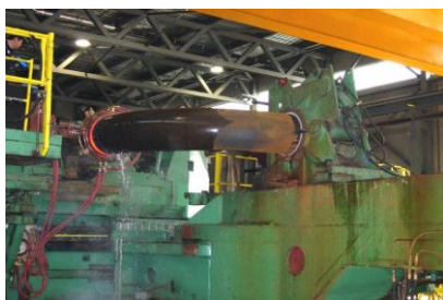
Fig. 1. Bending process of the pipe using induction heating
