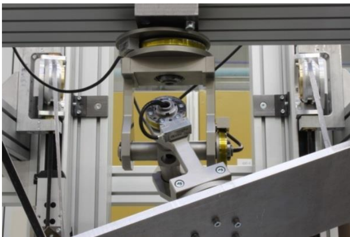
Fig. 1. The QuadroSphere tilting mechanism – central spherical joint with sensors
